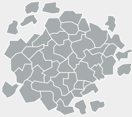
Polycrystalline structure enables self-sharpening
