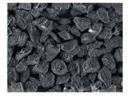
ULTRA-SOL® "M" aluminum oxide slurries feature high purity, tightly controlled particles to provide fast removal rates and good surface finishes.
