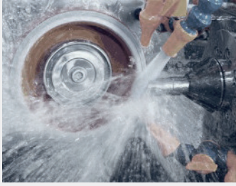
VECTOR HTR is useful for keeping glass or silicon off cast-iron plates.
