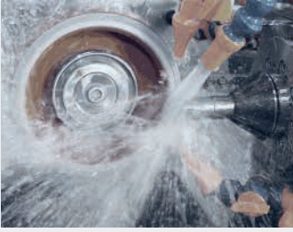
CHALLENGE grinding fluids improve the quality and consistency of the cut, while also prolonging diamond wheel lifetime.
