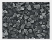
ULTRA-SOL® diamond alumina blends are excellent polishes on hard substrates such as SiC and also may IR and optical materials.
