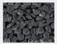
ULTRA-SOL® milled alkaline alumina suspensions feature high purity, tightly controlled particles to provide fast removal rates and good surface finishes.
